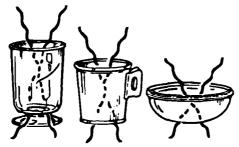
**Microwaves** pass through most glass, paper, and plastics without heating them so food absorbs the energy. Microwaves bounce off metal pans so food does not absorb the energy.
