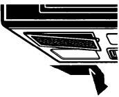
2. To remove grease filters, slide each filter to the side. Pull filters downward and push to the other side. The filter will drop out.
