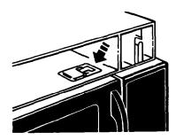
4. Remove bulb holder mounting screw.
