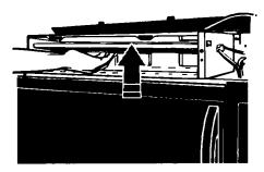
7. Lift the back of the charcoal filter. Slide the filter straight out.
