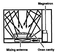
A magnetron in the microwave oven produces microwaves. The microwaves move into the area under the oven floor. There they bounce off the mixing antenna into the oven where they contact the food.
