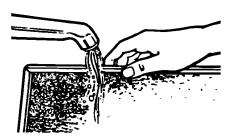
Soak grease filters in hot water and a mild detergent. Scrub and swish to remove embedded dirt and grease. Rinse well and shake to dry. Do not use ammonia or place in a dishwasher. The aluminum will darken.
