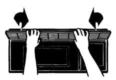
Slide the bottom of the vent cover into place. Push the top until it snaps into place. Replace the mounting screws. **10. Turn** the power back on at the main power supply.
