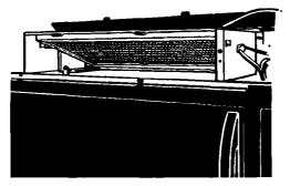
**8. Slide** a new charcoal filter into place. The filter should rest at the angle shown.
